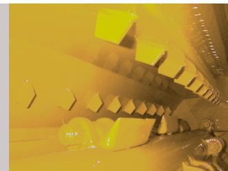
Rotorshaft, hammer knives and recutter blades
